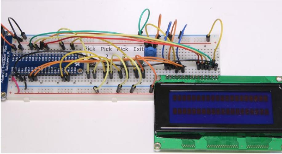
**Figure 4-12.** Physical setup for the automated Nim game
