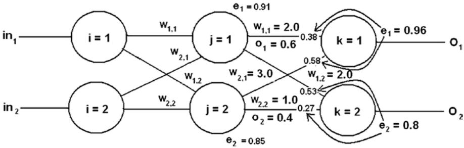
**Figure 8-23.** Example ANN used for manual calculations
