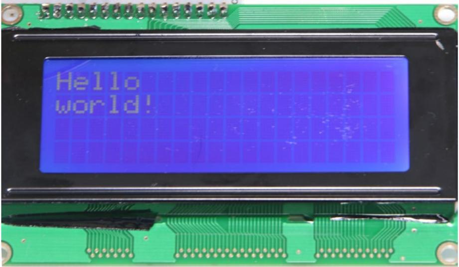
**Figure 4-14.** Result of running the `char_lcd.py` program
